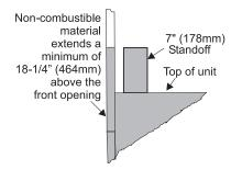
Install Top Standoffs & Side Nailing Strips before unit is slipped into position. See the "Unit Assembly Prior to Installation" section for assembly details.
